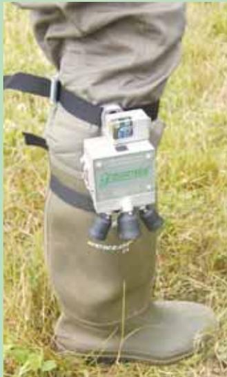
**Mounted on top of boot, monitor uses ultrasound sensors to automatically measure and track grass growth.**
