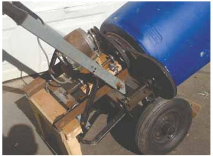
**An electric motor belt-drives the mixer barrel. Three belts reduce barrel speed to 25 rpm’s.**
