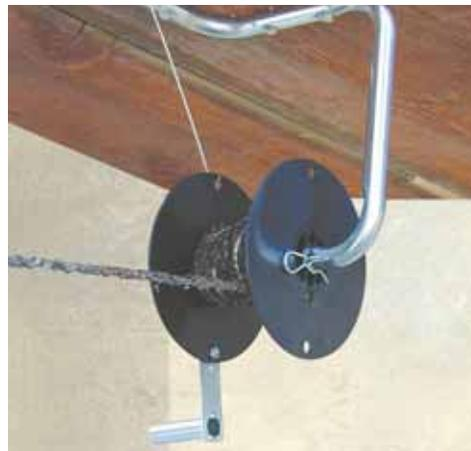
**Reel-to-reel system stretches 1/4-in. glue tape about 6 in. below the ceiling. Once the tape is full of flies you crank it up to expose fresh tape at the other end.**
