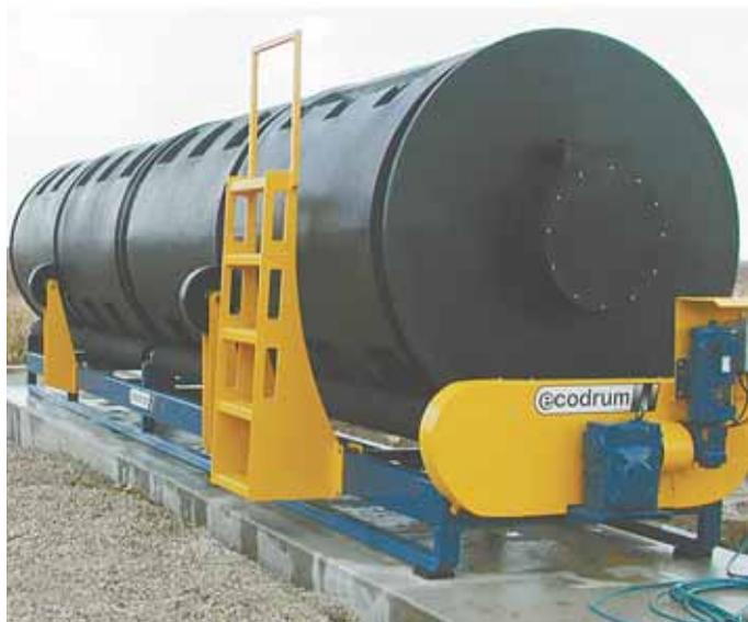
Ecodrum composter uses a molded polyethylene barrel to break down swine and poultry carcasses fast and completely.
