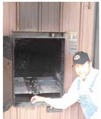
Edward Jewell says his new grate for Central Boiler wood furnaces is designed to burn wood more completely and results in less material to clean out.
