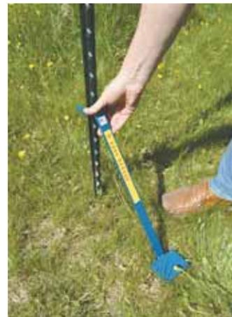
post. As the post emerges from the ground, the top of the T-post Badger ratchets down the knobs of the T-post.
