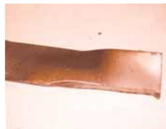
Unsharpened "finger" at end of blade knocks stones out of the way and acts like a hook to pull grass into blade.
