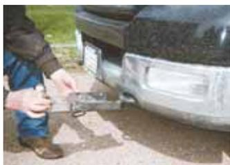
Hitch slips over pickup's tow hook. A steel pin inserts from underneath through the tow hook.
