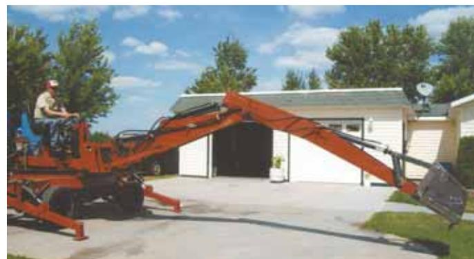
A hydraulic pump belt-drives a pair of tubeless rubber wheels that ride inside around top of turntable to rotate boom. Bucket can reach out 16 ft. and down more than 10 ft.
