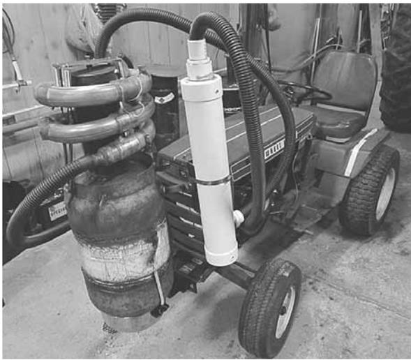
Jeff Davis runs his Wheel Horse garden tractor on charcoal, modifying a 30-lb. propane tank to make the burner unit. Gas runs through two 2-ft. long, 4-in. dia. pvc pipes.
