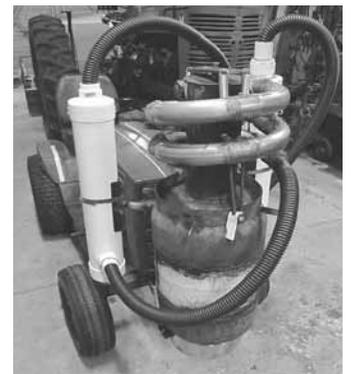
Pvc "filter" pipes are connected in series, mounted on each side of the tractor.
