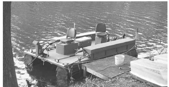
**A pickup ladder rack forms the frame of this "fishing boat" pontoon built by Robert John. It floats on six 55-gal. plastic barrels and has two 12-volt trolling motors.**
