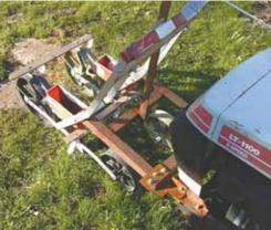
Victor Riggen mounted 2 Earthway planters spaced 12 in. apart on front of his garden tractor. Planters are raised and lowered together with a manual lever.
