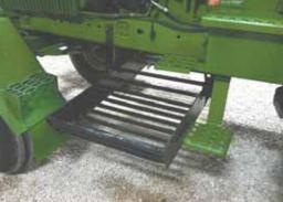
Heavy-duty rock carrier mounts under Deere 4440's frame behind the front wheels. Pipes are spaced 2 in. apart to allow any dirt to drop out onto the ground.
