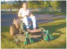
Suspension kit lets you drive zero-turn riding mowers faster and with fewer bumps. It works on new or used mowers without front end suspension.
