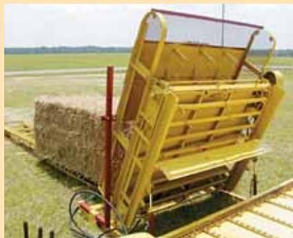
**Separator head drops loose hay onto conveyor, where it feeds into small square baler. Bale elevator carries bales away for stacking.**
