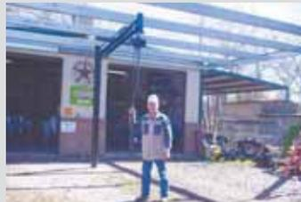
inside the shop through the doors. I just grab a chain and swing the hoist in either direction. The 12-ft. long I-beam on top of the hoist pivots on 3/8-in. bearings and can lift up to 2,000 lbs.
