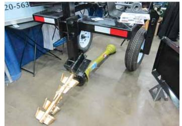
Twister Trencher consists of a pto-driven hardened shaft fitted with a series of cutting blades that penetrate dry, hard-packed soil.
