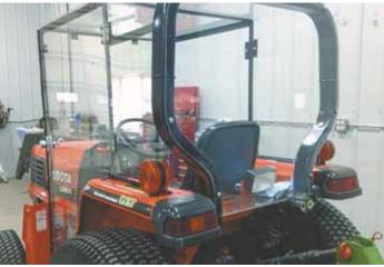
Blackburn bought the plexiglass in 4 by 8 sheets and cut everything to fit. He used 1-in. steel tubing to make a 4-section frame and attached the back piece to the rollbar.
