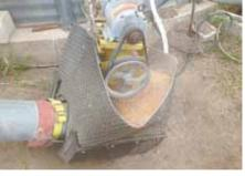
AugerBox is designed to enclose a discharge auger and funnel any flying grain down into the transport auger, minimizing waste and clean up.
