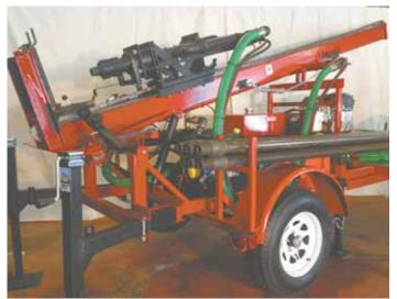
Compact Aqua Bore well drilling rig is small enough to be carried in a pickup bed or towed on a trailer by a pickup or small tractor.
