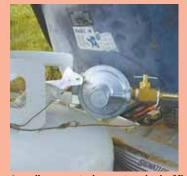
A small propane tank mounts on back of Bodell's lawn tractor, along with a regulator and hose that leads to the tractor's air cleaner.
