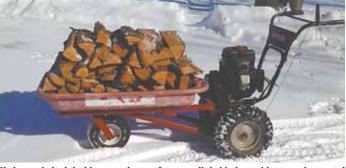
Bledsoe unbolted the blower and auger from a walk-behind snowblower and mounted a small wagon box in their place. It rides on a single caster wheel.
