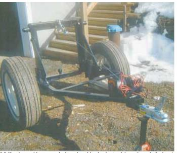
Phil Harris uses his power winch-equipped log hauler to pick up the end of a log. A removable crossbar on back with a ball hitch can be used to tow a trailer.
