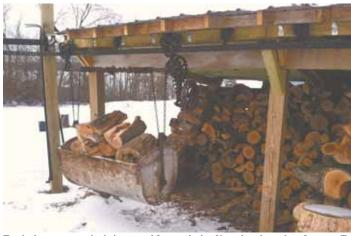
Tracked manure carrier brings wood from a shed to Norenberg's outdoor furnace. To mount the track, he extended the eave on his woodshed and mounted the rail beneath it.
