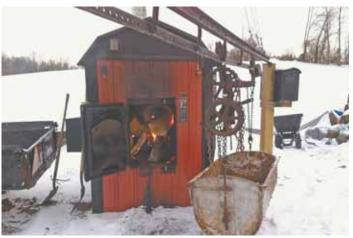
A chain hoist is used to raise and lower the carrier for easy loading and unloading.
