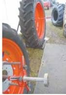
System uses a laser attached to the wheel rim to make sure big tractor Haweka AG from tires are aligned, reducing wear and Germany makes tire lowering fuel consumption.
