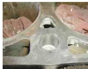
**Above "before and after" photos show how Lock-N-Stitch threaded inserts were used to repair a cracked Cat engine block.**
