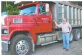
**Ron Peck's 1995 Ford dump truck has a gross vehicle rating of 75,000 lbs. and a load rating of about 23 tons.**
