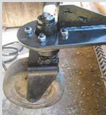
spindles and hubs are much stronger than the factory ones on the mower. The photos show 'before and after' photos of the conversion.
