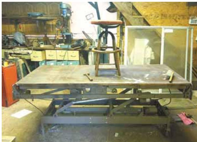
**Jim Borden converted an old hospital bed into an adjustable height workbench. He uses a foot pedal to raise and lower the unit anywhere from 16 to 34 in.**
