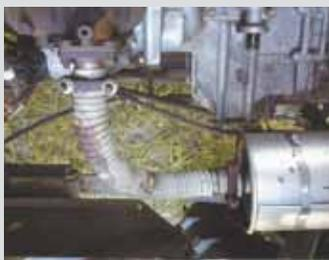
**Lloyd R. Lucas, High Springs, Fla.:** "I was going through a lot of air filters on my Kubota UTV until I made this change. I ran a long piece of pvc from the filter up through the roof of the vehicle. Pulls in clean air. Big improvement and I'm running with a clean filter much longer."
