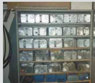
parts. Cut out one side of the can and then build a simple cupboard with shelves as deep as the cans and as wide as you want. The distance between the cans should be about 1 1/2 the depth of the cans so that you can overload them and still see what's in
