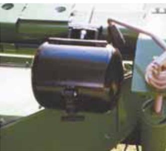
"Propane bottle" toolbox is bolted on back of Janssen's Deere mower-conditioner. Metal pins and pipes welded on inside the bottle are used to keep tools in place.
