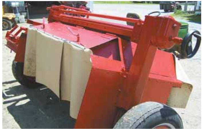
Belting at the front and back of machine keeps the churning compost contained.
