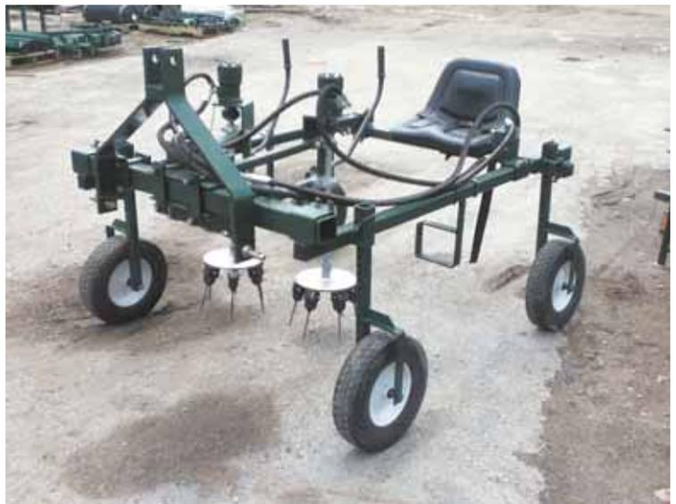
Willsie Equipment's 3-pt. mounted Hydroweeder allows a person to sit and operate rotating digging heads around plants.
