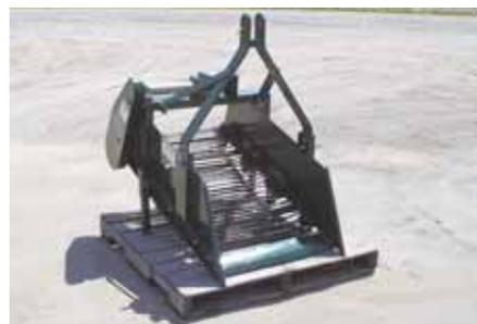
Hitch Digger digs up row crops for harvest, and the Electric Batch Washer quickly cleans vegetables.
