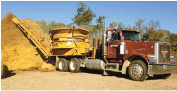
To beef up their custom hay grinding operation, Bryant Noot and his father Jay converted a pull-type Mighty Giant tub grinder into this truck-mounted unit.
