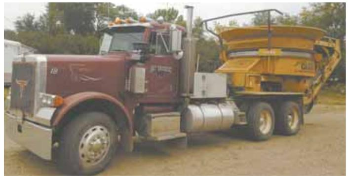
They repowered the semi tractor with the 410 hp Cummins diesel that originally powered the grinder, so now the engine supplies power for both the truck and the grinder.
