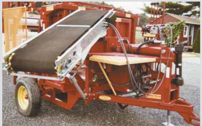
Bale Wrapper lets you wrap small square bales in plastic to make haylage. Bales can be loaded into machine using a 6-ft. rubber-belted conveyor (optional).
