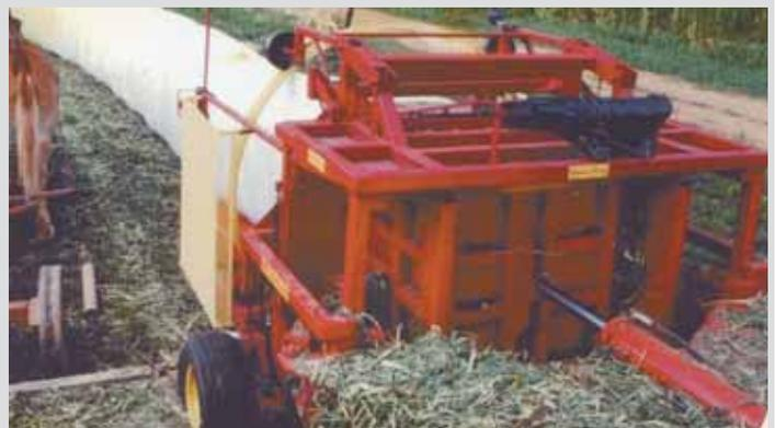
Machine compresses 8 small bales together from the top and sides, then pushes them through a 4-ft. sq. chamber which leads to the wrapper.
