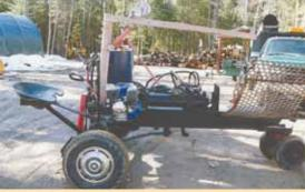
a gravel screening plant and cut it down to size. My only expense was the \$100 I paid for the Honda clone engine."
