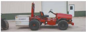
Dale Seaquist custom-builds forklifts for orchard use by modifying 3/4-ton, 4-WD pickups with special lift forks and an air bag suspension system.
