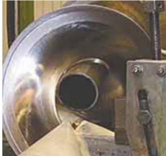
**Princeton Flighting Corp. repairs augers with conventional helicoid flighting. Its Super Edge flighting is up to 50 percent thicker where the greatest wear occurs.**
