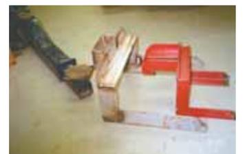
**One end of hangar slips over pads on lift.**
