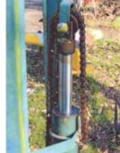
Forklift mounts on a snowplow mounting bracket on Gorge's Deere garden tractor. Forks are attached to a carriage that's raised up or down by a hydraulic cylinder.
