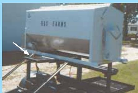
Instead of spending the money for a new truck-mounted hay cube feeder, Robert Sutterfield bought a used 3-pt. mounted model and rebuilt it. Arrow points to small solar panel that powers the feeder.
