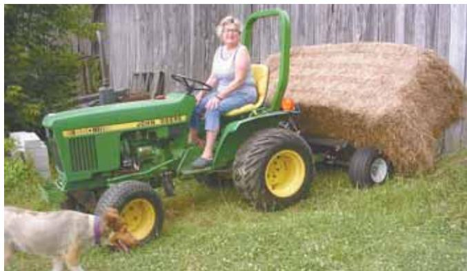
Lonnie Fast recently modified his Hay Baby, designed for ATV's to move big round bales, to also work on compact tractors with 3-pt. hitches.
