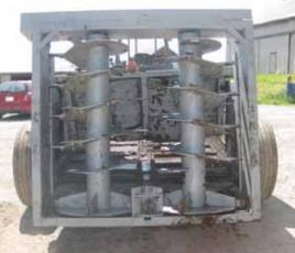
The Bowmans iobbed out the construction of the beaters to an auger specialist. Flighting on the 36-in. dia. beater was made from 3/8-in, steel.
