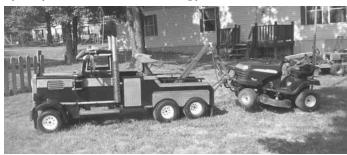
Stockton's 9-ft. wrecker has air intakes on the sides and a forward tipping hood. The metal cab and body were fashioned from a 300-gal, fuel tank.
