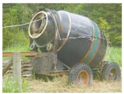
Russell Casperson used the drum off a portable cement mixer to build this electricpowered, 6 cubic yard composter.
