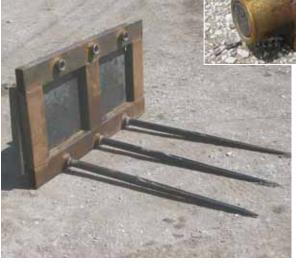
To mount bale spears, Schweppe pushes spears tĥrough welded-on bushings and out the back, then inserts a 1/2-in. bolt through holes already in each bushing.
