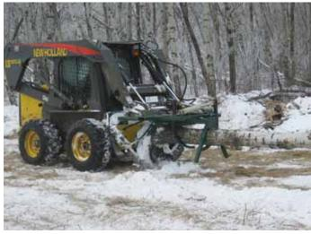
After tree is cut off, St. John lowers it to the ground for stacking or to cut up with chainsaws.
