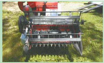
Mini combine has twin cutter bars - one mounted on the gathering reel to clip the grain heads, and the other mounted near ground level for cutting straw.
