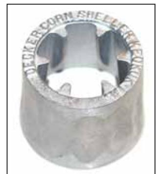
To use the mini sheller, you twist the ear through the collar and let sheller's 6 ridges rub the kernels off.
