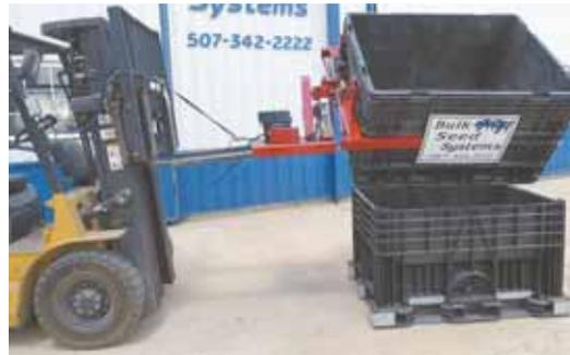
Seed box flipper slides onto standard forklift forks. Arms powered by an electric actuator open and close to grip seed box.
