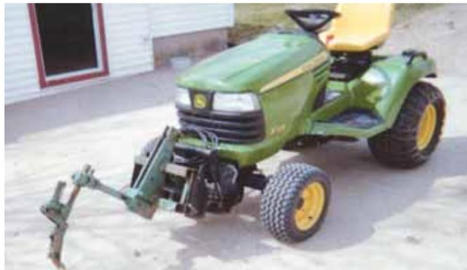
Garden tractor turf cutter uses a shank off an old cultivator.
