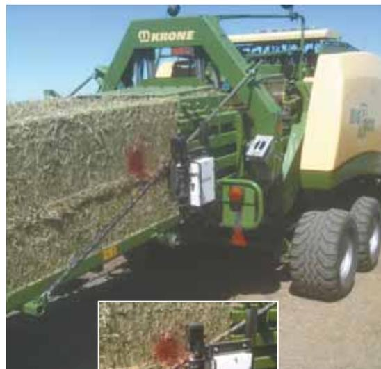
Baler-mounted moisture meter uses microwave technology to detect slugs of wet hay inside big square bales.
