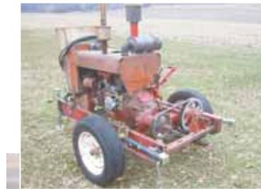
Larry Ristau modified an old combine engine to run on propane, turning it into a stand-alone power source that he uses to power his grain dryer. The pto shaft and bearings are from an old Allis Chalmers tractor.
