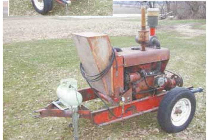
valve to the mini-tank and vapor feeds into the carburetor to start the engine.
