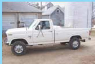
Burning a little LP makes Larry Ristau's 1985 Ford F-350 diesel pickup run better. An 80-lb. LP tank mounts in the bed.
