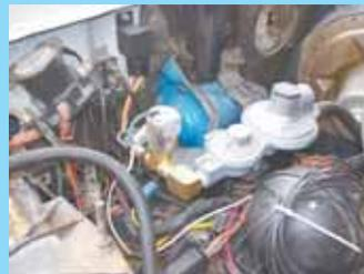
To add LP to the air flow, Ristau uses a 2-stage regulator that comes with an adapter plug to fit LP tanks. The regulator is installed in the engine compartment where it delivers gas to a solenoid valve.
