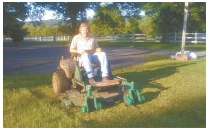
Suspension kit lets you drive zero-turn riding mowers faster and with fewer bumps. It works on new or used mowers without front end suspension.
