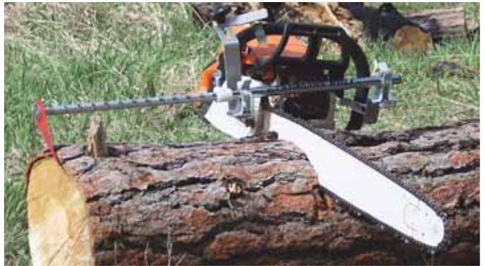
The Chainsaws Rule allows you to measure the wood as you cut it. Telescoping rod has 1-in. markings on it and a red aluminum flag at one end.
