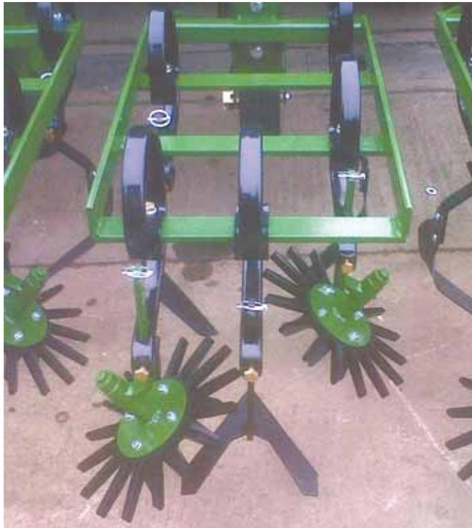
Fingerweeder spoked wheels mount at an angle to the cultivator shaft, and use flexible fingers to break up small roots on freshly germinated weeds.
