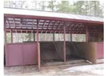
Joseph Baril’s 25-ft. long compost shed is divided into a series of 5-ft. wide bins fitted with swing-out doors. Baril dumps material almost daily into one of the bins.
