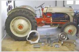
Photo shows parts included in overhead valve conversion kit for N-Series Fords.
