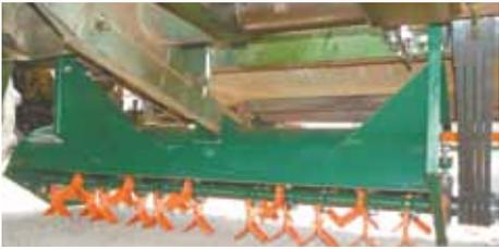
Chop Rite stalk chopper mounts under New Idea pull-type corn pickers and is belt-driven off the picker gearbox.
