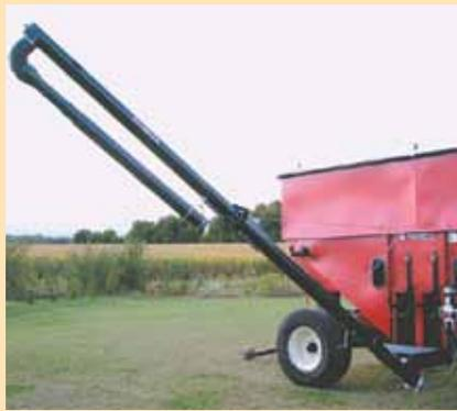
New-style 18-ft. auger can reach out 28 ft. in front and 55 ft. from side to side to fill planters and grain drills. Auger folds down within the length and height of most gravity boxes.
