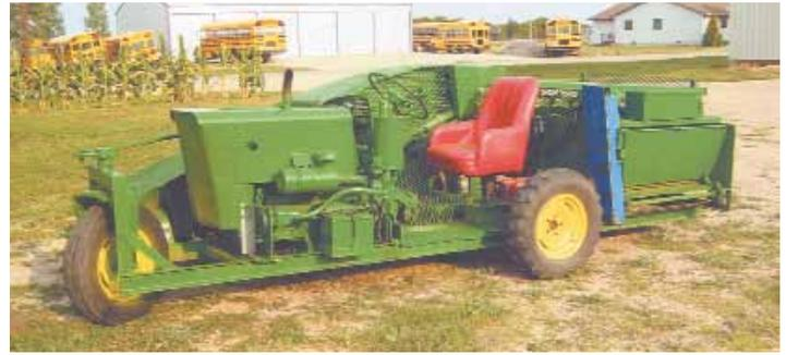
The operator rides in comfort on a cushioned chair while steering a single front wheel. Foot and hydraulic controls are within easy reach.
