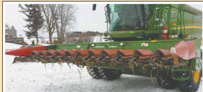
Forde made this “rowless” narrow-row cornhead to harvest corn planted in 12-in. rows. He started with a 12-row, 20-in. IH cornhead, cutting off the steel plates for mounting the snouts so he could move the row units closer together. He added a 6-in. wide divider with a turned up point (below) between row units to help feed stalks into header. Header was used with and without snouts to harvest corn, running in any direction through field.
