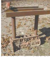
Lengths of pipe, inserted into engine block cylinder holes, support a tabletop made from sections of a trailer ramp.
