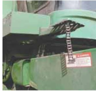
**Bob Lounsberry, Columbus, N.J.:** "I used to have to hunt all over whenever I needed the header drive coupler chain for my Deere combine. I solved the problem by attaching an S-hook to the bottom of one of the steps to the cab. Now I always know where the chain is hanging."
