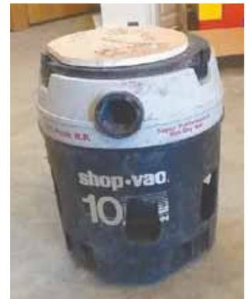
Converted 10-gal. Shop-Vac has several feeding ports cut into the side.
