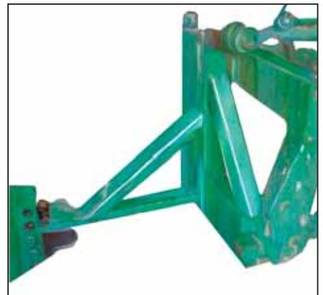
Drawbar on home-built, 3-pt. mounted extension lift can be raised up to 2 ft.
