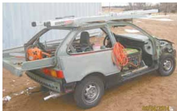
Drawdy removed car's doors, seats and rear hatchback, then built a plywood platform on the passenger side and on back. Wooden rack on top is used to haul a ladder or other cargo.
