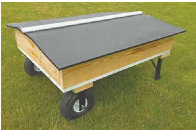
Wheeled mineral feeder has a cover made from 1/2-in. floor mat. Livestock lift the cover with their nose.
