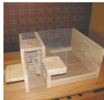
“Walk in” bird trap measures 18 by 16 in. and is 8 in. high. It’s made from wood and 1/2-in. hardware cloth.
