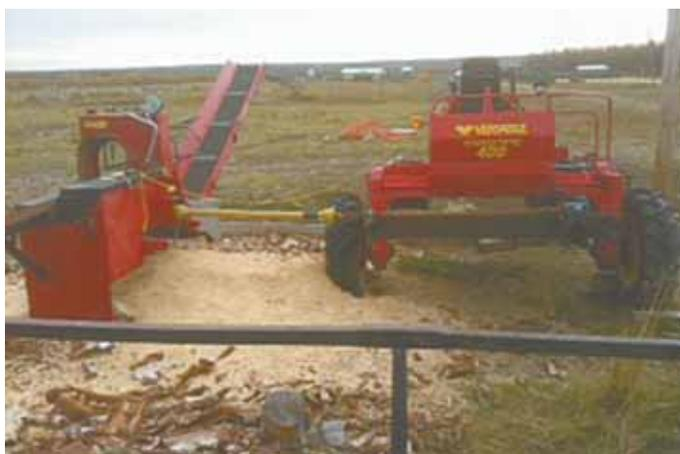
Allan Ritchie converted an old Versatile self-propelled swather to use as a pto power source for his firewood processor.
