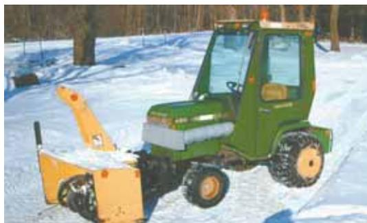
Ron Nikolai made a cab heater for his Deere 420 garden tractor, which is equipped with a front-mounted snowblower. It captures heat from the front of the tractor and shoots it around the side and back into the cab.
