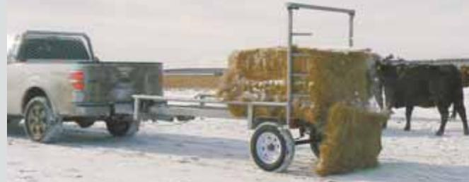
Power Rack bale feeder is equipped with retaining "fingers" that release flakes from bale as it's pushed backward on rack.
