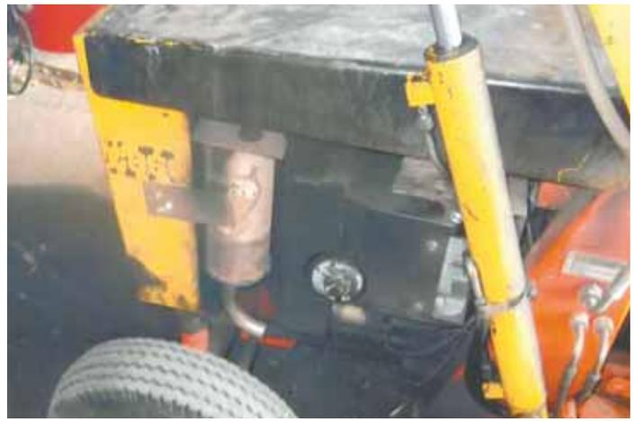
Home-built muffler was made by cutting 16 in. off a 4-in. dia. grain auger and welding a length of flanging inside. A curved exhaust outlet is bolted on at bottom.
